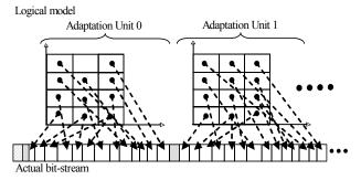
Fig. 1 Bit-stream example showing two adaptation units with 3x4 logical hypercubes in each. Light-shaded and cross-hatched segments correspond respectively to *update* fields and segments that are neither included in logical units nor are update fields.
