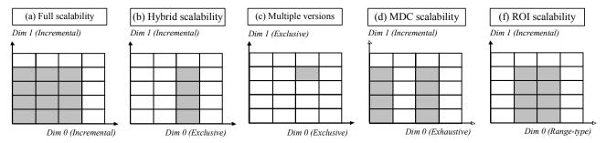
Fig. 2 Various types of dimensions of the logical hypercube model and scalabilities derived from their combinations
