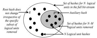
Fig. 4 Flexible partitioning of logical unit hashes
