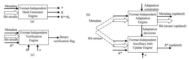
Fig. 5 Format Independent Authentication Components, all driven by metadata
