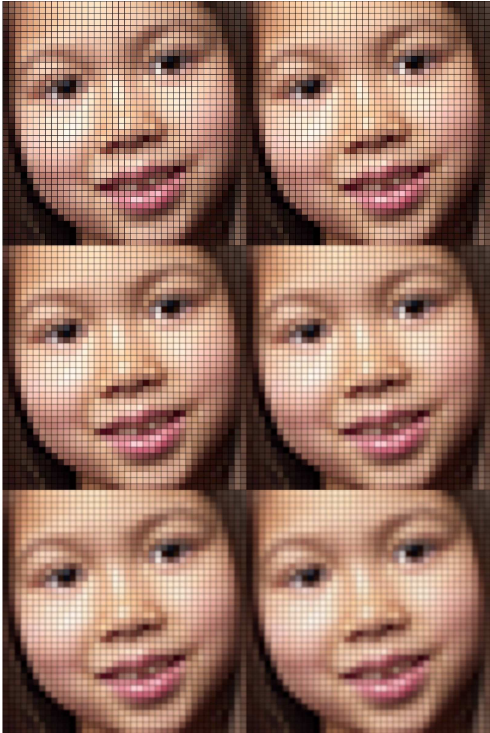
Figure 2.5: Examples of images generated with a projector with 90% aperture ratio, and different anti-aliasing Gaussian filters. The filter parameters are, from left to right, and top to bottom, \sigma = 0, 0.04, 0.08, 0.12, 0.16, \text{ and } 0.2 .
