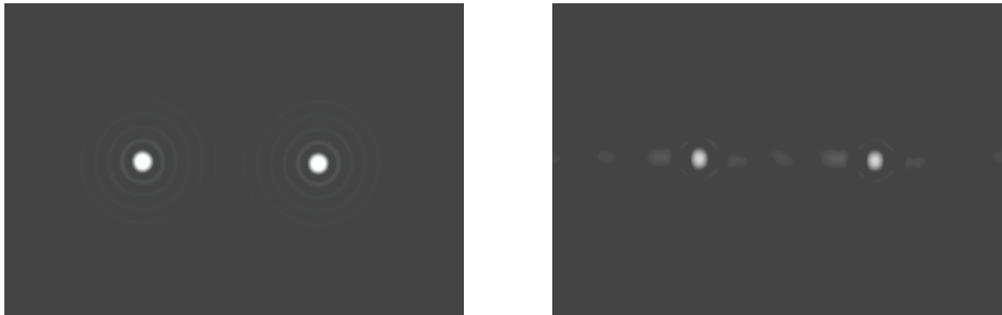
(a) In the absence of the wire grid (WG) in Fig. 2, each image spot exhibits an Airy pattern due to the finite diameter lens ( L ) acting as a low-pass filter.
