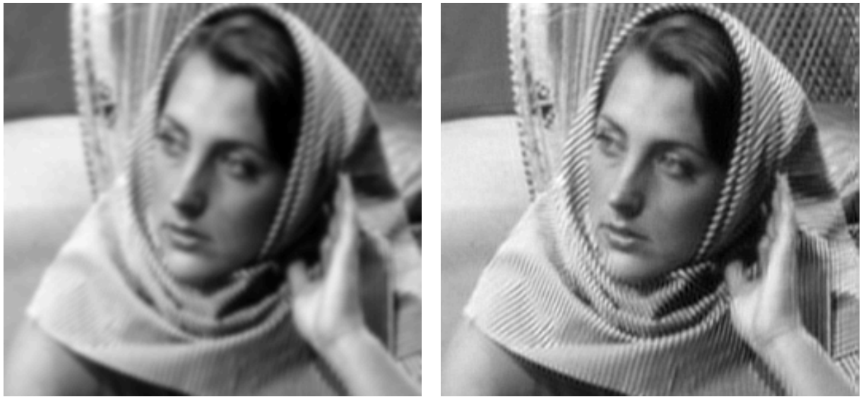
Figure 25: Left: Blurred BARBARA after applying a 5-tap Gaussian blur. Right: Sharpened BARBARA using LUTs that were trained on blurred LENA using 8x8 over-complete DCT.
