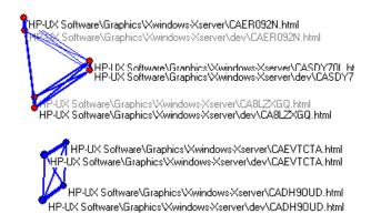
Figure 7: Without special handling for identical files, the number of similar file links multiplies.
