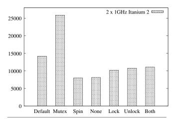
Figure 3. Msecs to copy 10MB/thread in 2 threads on 1GHz Itanium 2
