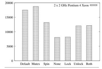
Figure 4. Msecs to copy 10MB/thread in 2 threads on 2GHz Pentium 4 Xeon
