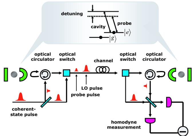
FIG. 1: (Color online). Schematic for the generation of spin-entanglement between two qubits at neighboring stations via homodyne detection discriminating between conditionally phase-rotated coherent probe beams.
