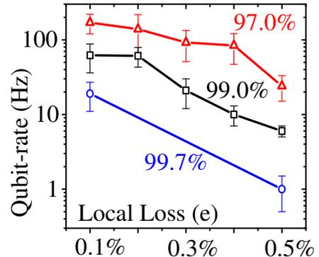
FIG. 3: (Color online). Achievable qubit communication results (in terms of qubit rates for different target fidelities) vs. local optical losses ( $\epsilon$ ). Each point corresponds to a single Monte-Carlo simulation of the nested purification protocol over 9 complete qubit teleportations; each point is the average difference in time between teleported qubit arrival times, and the error bar is the standard deviation.
