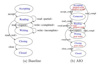
Figure 3: State machine for handling a single connection
