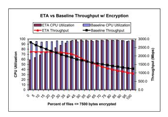
Figure 5: Peak Throughput and CPU Utilization with an Application Workload
