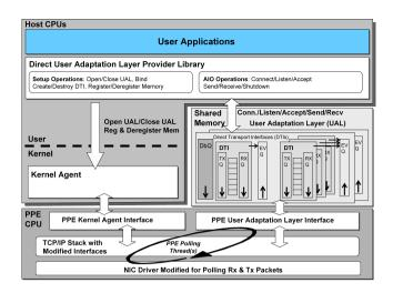
Figure 1: DUSI/ETA PPE Software Architecture
