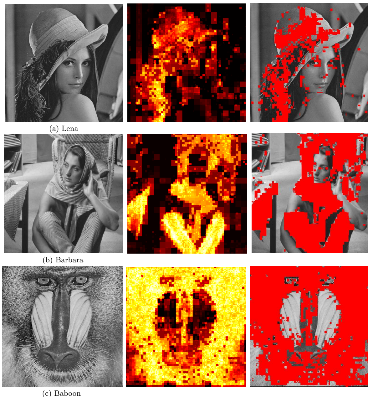
FIG. 8: Examples of texture detection. Likelihood measures were thresholded to obtain the rightmost images.
