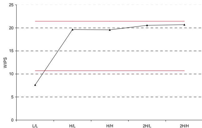
Figure 9. System throughput (WIPS). Lines above and below the curve demarcate bounds on the range of acceptable operating throughput based on ideal TPC-W performance as a function of the number of EB's.
