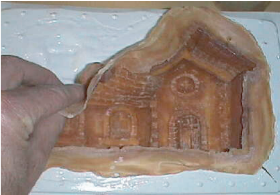
Pour plaster over a spatula; add reinforcement, followed by more plaster; then mark cast with ID and arrow pointing North.
