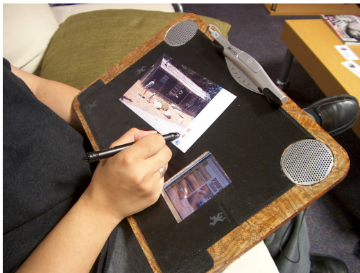
Figure 6. Stand-alone active-photo appliance, with speakers and exposed iPAQ screen.
