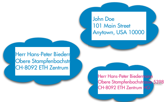
Fig. 1. Mailing label on a VDP piece. The cloud indicates that the area surrounding the address is colored. In this example the designer has chosen to print the address in the same color as the surround. While this can work well on short US addresses, it fails for example on addresses in German, where critical information for the delivery of the mail piece becomes invisible. When a contrasting color is chose to print the address, critical information is still readable to the letter carrier.
