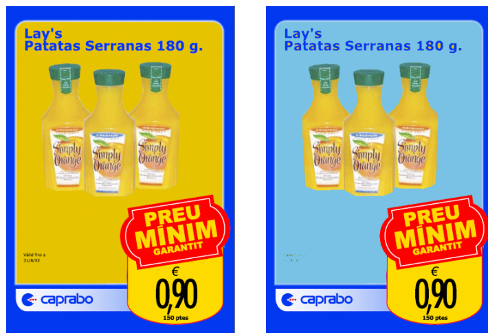
Fig. 2. In this VDP example, in-store advertisements for sales promotions are printed by enumerating information from a database and placing it on a rich template, whose main color is chosen to attract customers' attention. When the image of an item happens to be of the same or a similar color as the background, the promoted item can “disappear” in the template.
