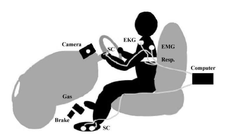
Figure 1: The subject wore five physiological sensors, an electrocardiogram (EKG) on the chest, an electromyogram (EMG) on the left shoulder, a chest cavity expansion respiration sensor (Resp.) around the diaphragm and two skin conductivity sensors (SC), one on he left hand and one on the left foot. The sensors were attached to a computer in the rear of the vehicle.
