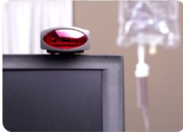
Figure 1: SAP Infrared Transceiver Located on Data Terminal Display
