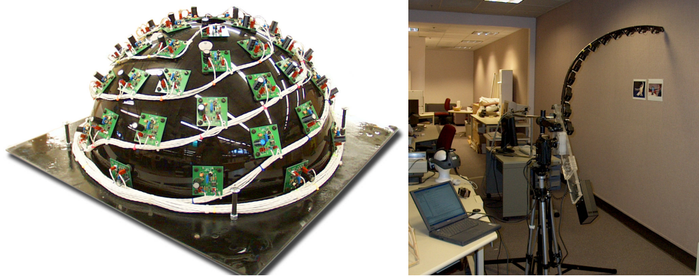
Figure 1: Dome and arm PTM capture devices
