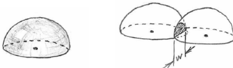
Fig. 7 Buildup on plane surface from: a) One dimensionless point. b) 2 points, intersecting at a knit plane.
