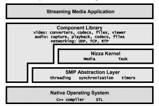
Figure 3. Implementation hierarchy. Nizza forms the middleware between the application and native OS. While the SMP abstraction layer keeps the kernel platformindependent, some modules in the component library (*e.g.*, camera drivers) must be device-specific. that traverse the Task graphs, keeping track of computational statistics such as mean latency and throughput.
