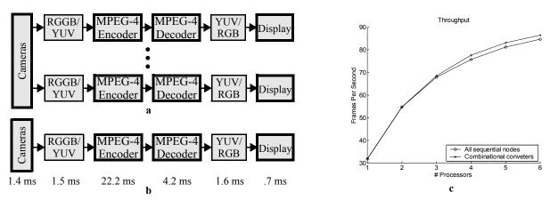
Figure 5. Video coding: (a) Model application, with sequential modules illustrated with a thick boundary. (b) Experimental setup showing mean module latencies for a single stream. (c) Plot for number of streams equals number of processors.
