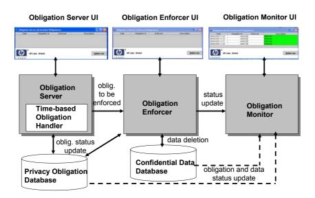
Fig. 2: Architecture of Current Prototype
