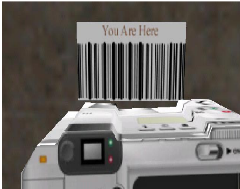
Fig. 8 Screenshot of the physical environment showing the simulated camera about to sense a bar-code (physical-hyperlink) to find location-specific services.
