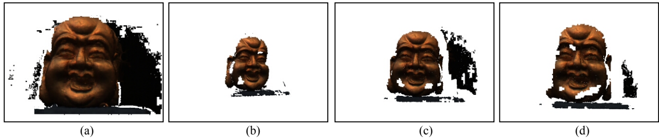
Fig. 7. "Buddha" image quartet using Blocks: (a) estimated projector's viewpoint; (b) synthesized view (0.5,0.5) from triplet 1; (c) synthesized view (0.33,0.33) from triplet 2; and (d) synthesized view (0.12,0.20) from triplet 3.
