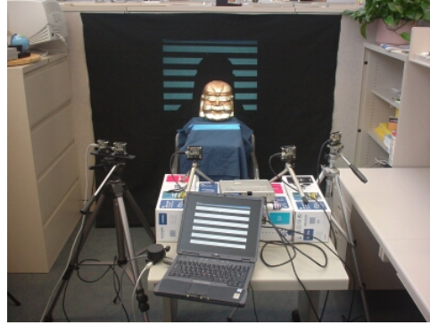
Fig. 4. The experimental LUMA system uses a DLP projector and up to four Firewire cameras connected to a notebook computer, shown here with one of the Stripes patterns illuminating the scene.
