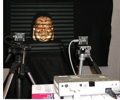
Figure 6. LUMA uses a projector and one or more cameras.
