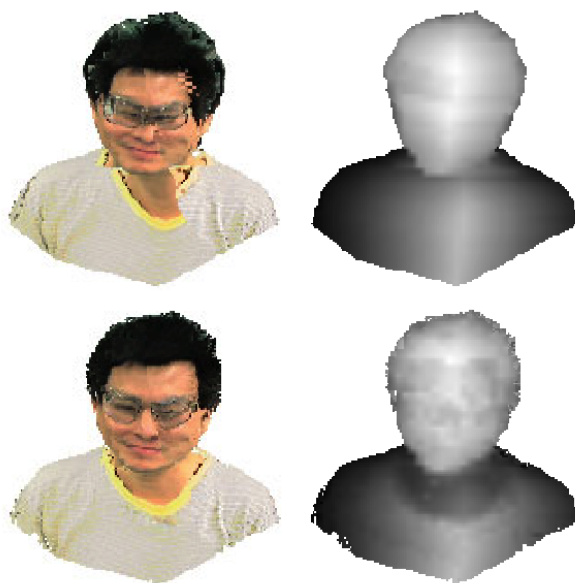
Figure 8. IBVH (top) versus IBPH (bottom). Texture-mapped model (left) and depth map (right).
