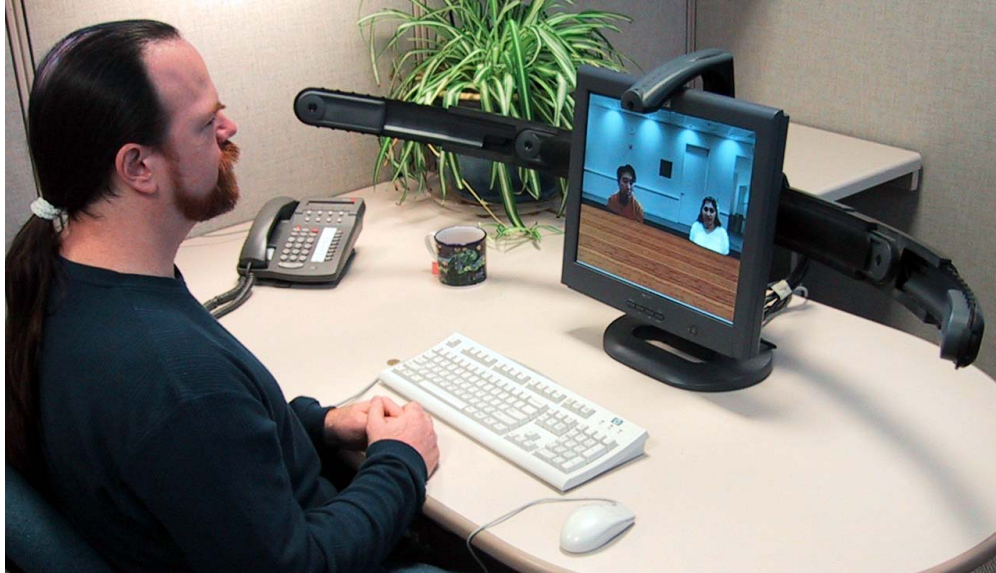
Figure 1. The Coliseum immersive videoconferencing system
