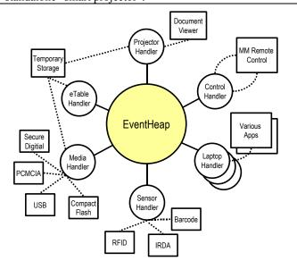
**Figure 2.** MeetingMachine Software Architecture Diagram. Whatever their hardware configuration, the software components (boxes) communicate through event handlers (smaller circles) to send events through the Event Heap (larger circle).
