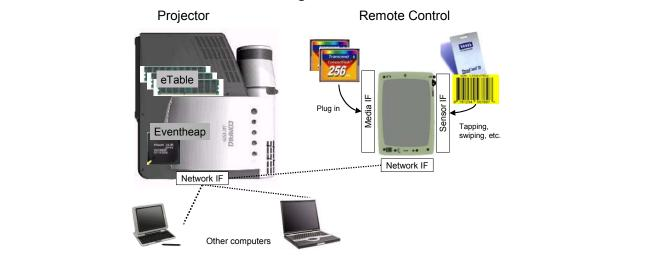
**Figure 1.** The MM consists of a projector with an embedded computer (or a separate appliance that can be connected to an unmodified projector), sharable temporary storage, ports for connecting storage media, and network interfaces.
