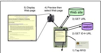
**Figure 5.** Operational sequence for converting a radiofrequency tag to a document in the MeetingMachine 1) User places RFID-embedded card on the ID reader, 2) MM contacts webid service with users' ID, URL is returned, 3) MeetingMachine gets web page, 4) Web page is projected...
