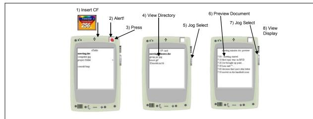
**Figure 4.** Screenshots from the Ubiwise simulator showing the operation of the MeetingMachine RemoteControl in transferring media from a CompactFlash to the eTable.
