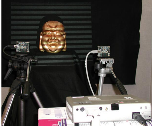
Figure 9. The experimental LUMA system uses a projector and one or more cameras.
