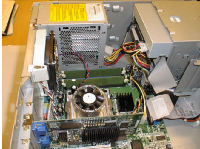
FIG. 2.2 The existing thermal management scheme utilized in the HP Vectra desktop computer.
