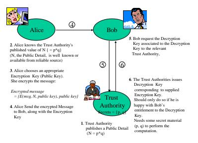
Figure 2: High-level IBE Interaction Model
