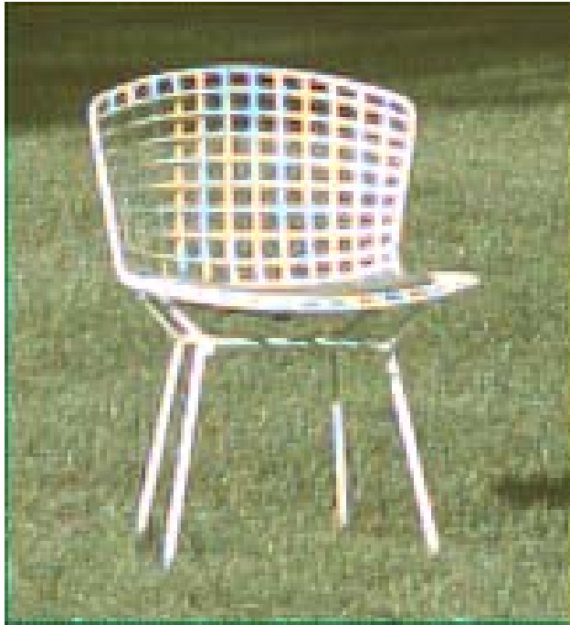
Figure 13: A demosaic image after applying the directional smoothing on each color band separately. Note the color artifacts near edges.
