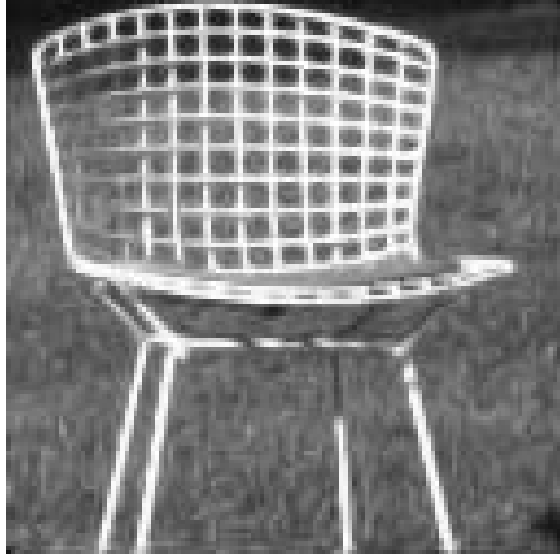
Figure 7: Directional interpolation of the green band taken by the Kodak DCS-200 camera. The interpolation was perform for all directions.
