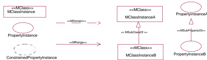
Fig. 6 Legend for instance of the meta modeling layer constructs to be used in developing the modeling Layer.
