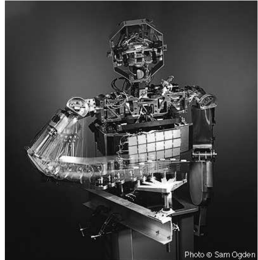
Figure 1: Picture of Cog turning a crank. The robot is using two shoulder joints and two elbow joints to create the motion of the crank.
