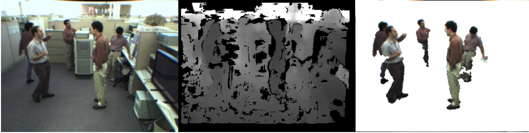
Fig. 4. Example camera-view input. From left to right, (a) Current color, (b) Current depth, (c) Foreground color. Unreliable (low confidence) depth data is shown in black.
