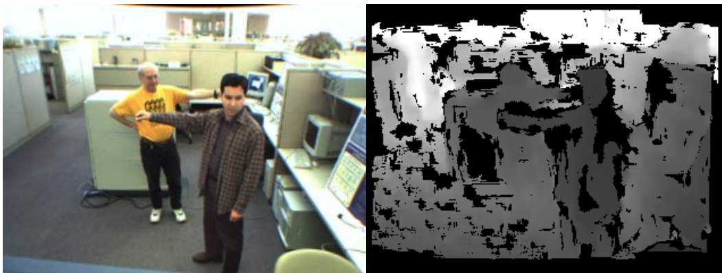
Fig. 1. Example of color-with-depth video input, obtained using the Point Grey Triclops camera [1]. In the depth image, brighter pixels indicate greater distance from the camera, and invalid (unreliable) depth data is shown in black.
