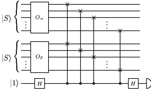
FIG. 1. A quantum circuit for the permutation promise problem.
