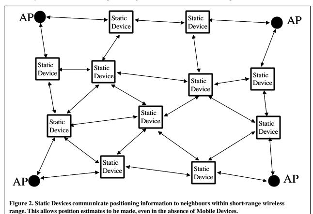
a) Initially Static Devices have no positioning information. A Mobile Device passes
