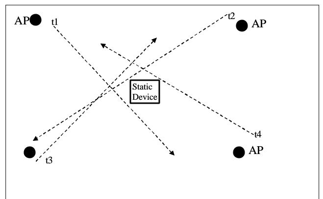
Figure 1. The dotted lines show the path of 4 Mobile Devices, which pass near to the respective Access Points at times t1, t2, t3 and t4, and progress towards to the Static Device, communicating position information with the latter. The times t1, t2, t3 and t4 could be separated from each other by hours or even days. Subsequently, this information can be communicated to another Passing Mobile.
