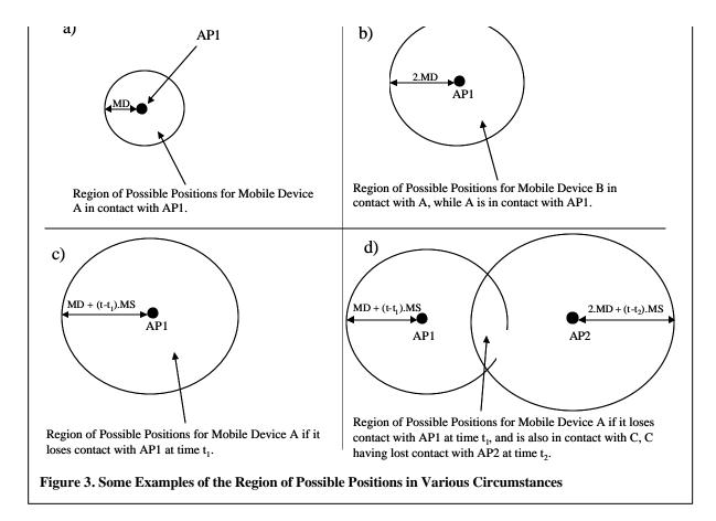
d) Suppose further that Mobile Device C last communicates with Access Point AP2 at time  $t_2$ , and then communicates with Mobile Device A at time t. Clearly,  $Dist(C, AP2) \le MD + (t - t_2)MS$ , and since C and A are now communicating,  $Dist(A, AP2) \le 2MD + (t - t_2)MS$  i.e. A is within a circle of  $2MD + (t - t_2)MS$ of AP2. However, it is also known from c) that  $Dist(A, AP1) \le MD + (t - t_1)MS$
