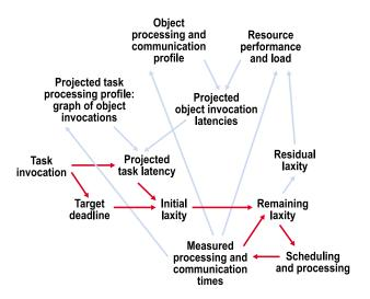
Figure 3: The Scheduling and Profiling Loop of the Decentralized Resource Management System.
