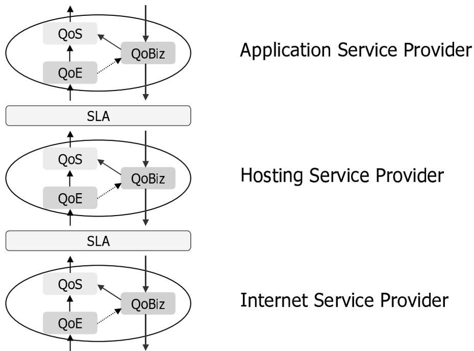
**Figure 3** XSPs: Service Level Agreements between service providers
