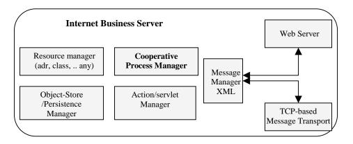
Figure 1: Architecture of IBS
