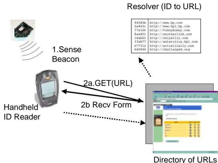
Figure 7. Resolver and directory selection for infrastructure-based physical registration
