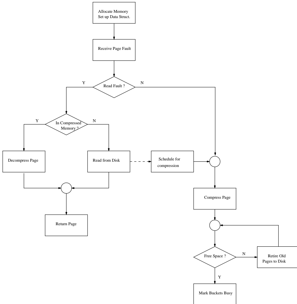
Figure 4: Flowchart of Memory Compression Algorithm
