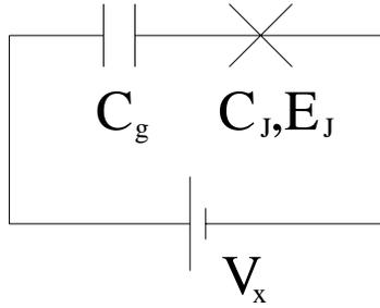
Figure 3: The circuit for a charge qubit. The voltage source  $V_x$  is connected through a gate capacitance  $C_g$ . This is shown as a single capacitor but in practice it may be composite (e.g.  $C_g/2$  either side of the weak link, in series.) The weak link (capacitance  $C_J$  and tunnelling energy  $E_J$ ) is simply denoted by X. In practice this can be a composite controllable weak link as described in subsection 3.6.
