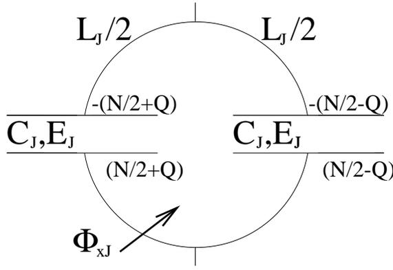
Figure 2: The circuit for a tunable  $E_J$ , which combines features of the model charge and flux qubits. Two weak links (with capacitance  $C_J$  and Josephson energy  $E_J$ ) are placed in a ring of total inductance  $L_J$  which is subject to an external flux  $\Phi_{xJ}$ .
