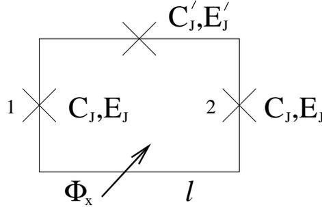
Figure 5: The multi-link circuit for a flux qubit. In practice the weak link with capacitance  $C'_J$  and tunnelling energy  $E'_J$  can be composite and controllable as described in subsection 3.6.
