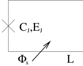
Figure 4: The rf SQUID circuit for a flux qubit. The weak link (capacitance  $C_J$  and tunnelling energy  $E_J$ ) is simply denoted by X. In practice this can be a composite controllable weak link as described in subsection 3.6.
