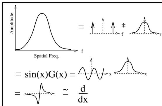
Figure 2: Shifted Gaussian is roughly a derivative operation
