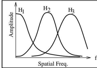
Figure 1: Qualitative description of filters modeling the *human contrast sensitivity* functions, in the spatial frequency domain
