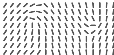
FIGURE 1 An example of the defect structures that arise when the model is started with the directors chosen entirely at random.
