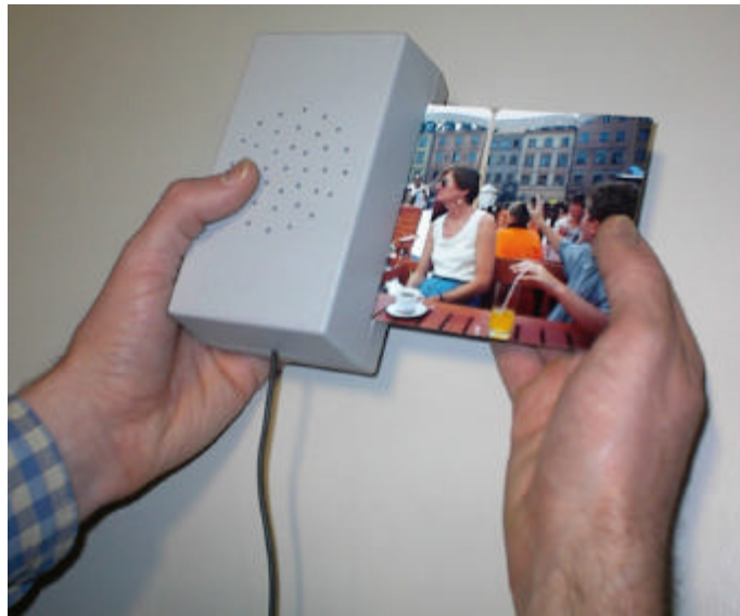
Figure 1. The audioscanner mock-up
