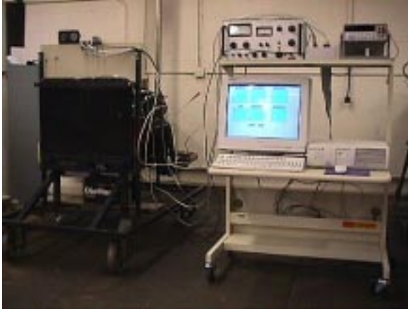
(a) Chevrolet V-8 engine mounted on a rolling frame and personal computer based instrumentation system.
