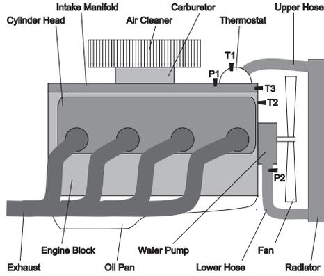
**Figure 3. Engine schematic with suggested sensor placement**
