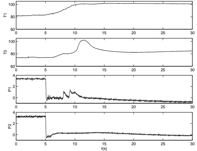
**Figure 5. Abrupt loss of coolant through punctured lower radiator hose**
