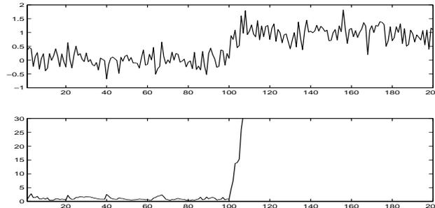
**Figure 2. Abrupt change detection in a unit step function with Gaussian noise ( $\sigma = 0.3$ ). The step occurs at  $x = 100$**
