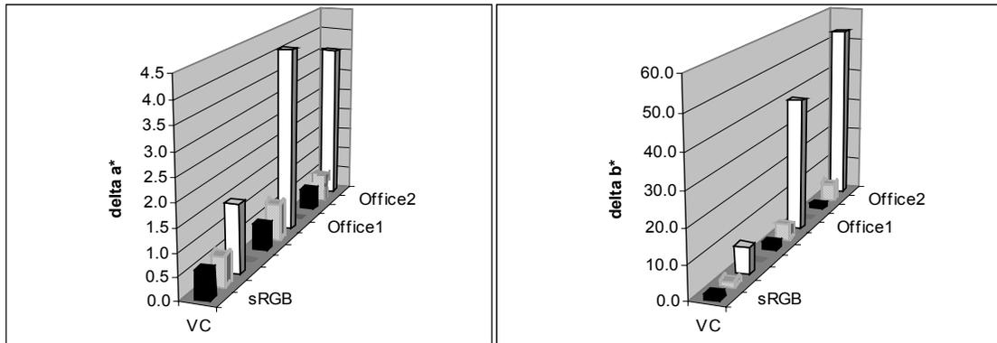
**Figure 8.** Plots of the difference between AWP results and the other VC measurements in CIELAB ( $a^*$ ,  $b^*$ ) plane. Black bars are difference from background measurement. Cross-hatched bars are difference from monitor WP, and white bars are difference from ambient WP. In all three viewing conditions the difference from background is much smaller. Note the scale of delta  $a^*$  plot versus that of the delta  $b^*$ . Most of the differences lie in the  $b^*$  direction.
