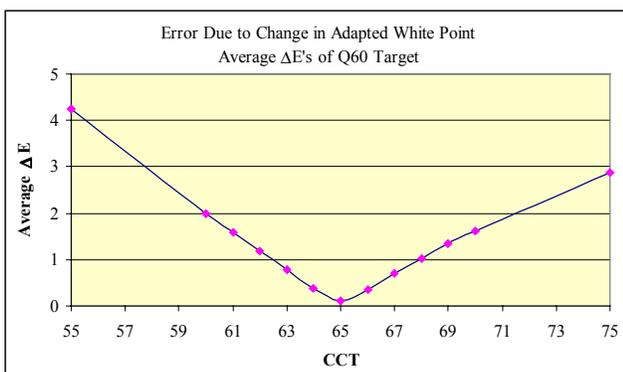
**Figure 1.** The 224 color patches of a Q60 target are measured under a D65 illuminant. We apply CIECAM97 whose chromatic adaptation point is set at another CCT, from D55 to D75, and measure the difference in output versus input. When the correct adaptation point, D65, is fed to CIECAM97, the  $\Delta E$  goes to zero, as expected, and the output matches the input. A 250-degree error in adaptation point causes  $\Delta E$  of 1.2.
