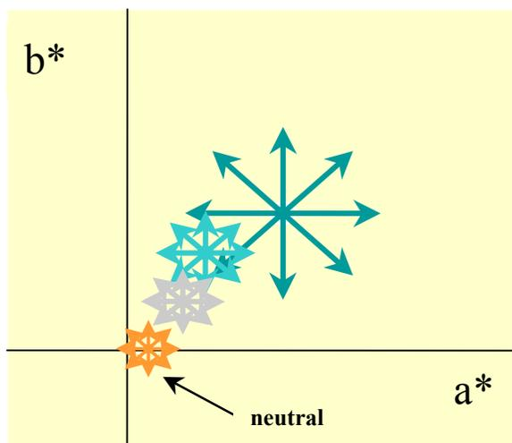
**Figure 3.** The process of converging to the neutral point. Every four screen-full of patches presented to the observer is one of the asterisk patterns above. The observer's four selections, one from each four screens, are averaged together and yield the center point for the next four screen-full of patches. This process will iterate and take us towards the observer's neutral point in the space. We stop when the standard deviation of the observer's four selections is less than 0.25 rms.
