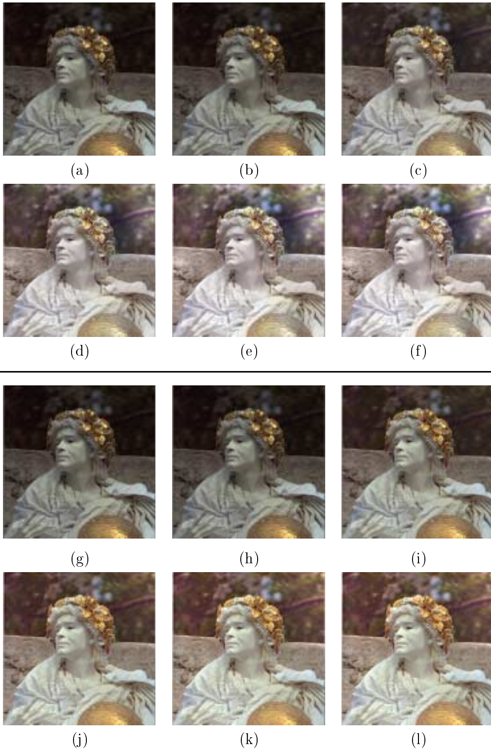
Figure 13: The influence of parameter \gamma (amount of illumination return). (a),(g) Original image, (b),(h) \gamma = 1 , (c),(i) \gamma = 2 , (d),(j) \gamma = 6 , (e),(k) \gamma = 24 , (f),(l) \gamma = 96 . Images (b)-(f) refer to processing of all RGB components separately, whereas images (h)-(l) correspond to processing of V component of HSV space only.
