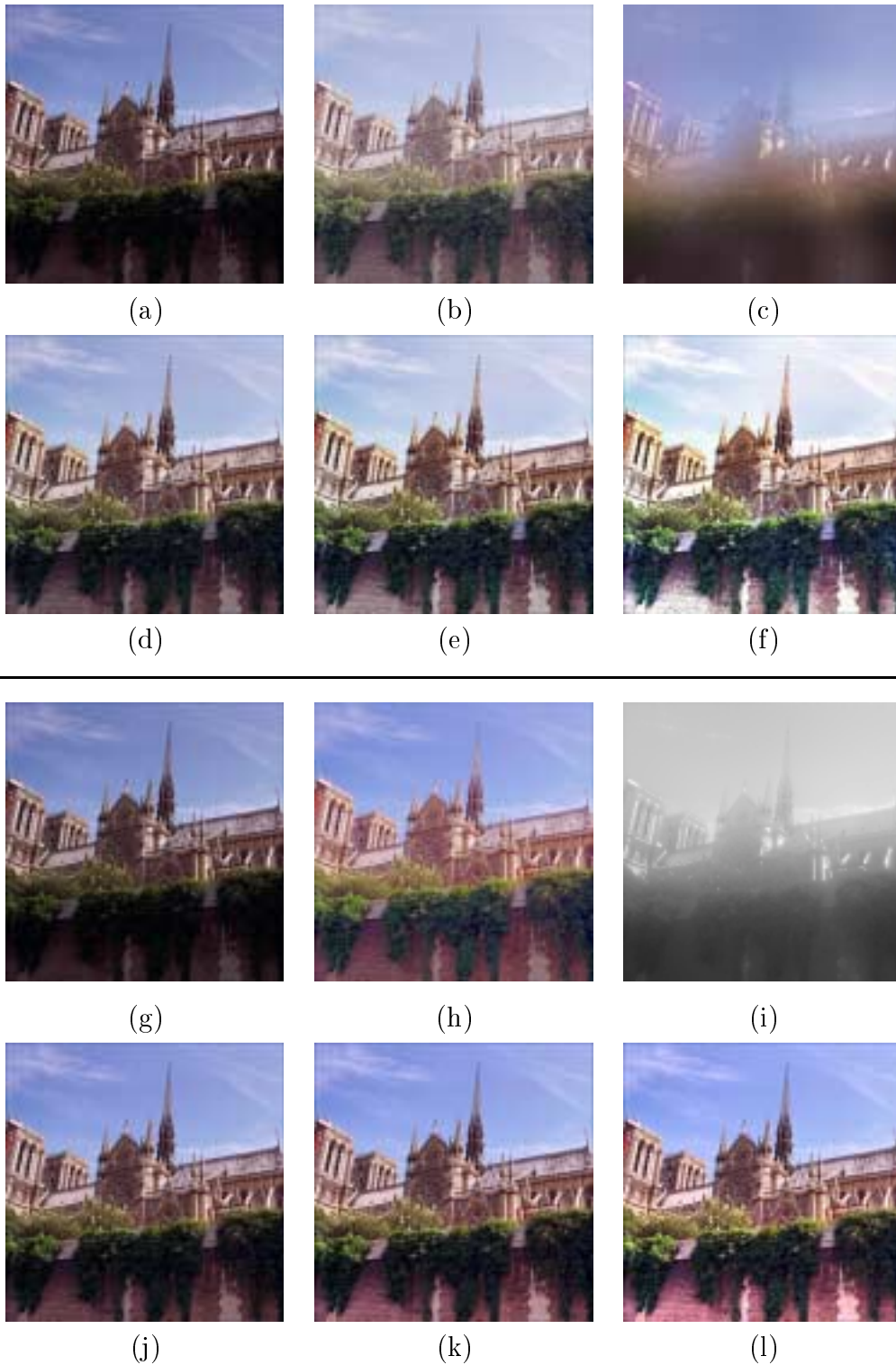
Figure 7: Example 4. Images (b)-(f) refer to processing of all RGB components separately, whereas images (h)-(l) correspond to processing only the V component of the HSV space. (a),(g) Original image, (b),(h) standard Gamma correction with \gamma = 2.2 , (c),(i) estimated illumination image, (d),(j) proposed alg. with \gamma = 2 , (e),(k) proposed alg. with \gamma = 4 , (f),(l) reflectance image (proposed alg. with \gamma = \infty ).
