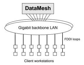
Even so, since the I/O capacity of each DataMesh node will be limited, the DataMesh will probably need on the order of 10–30 taps onto the 10 Gbit LAN, and FDDI may still be used to hook onto a backbone LAN using the multi-Gigabit hardware, partly for cost reasons, partly because FDDI networks will already be installed. In any case, availability considerations will also encourage the use of multiple LANs even if a single one could handle the traffic.
