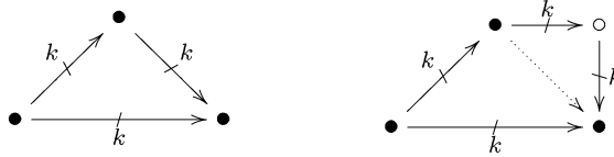
Fig. 2 Example of how to use a bypass node. In the graph on the left, each edge is duplicated k times and clearly \chi' = 3k . However, using only one bypass node, we can perform the migration in \Delta = 2k stages as shown on the right. (The bypass node is shown as “o”)
