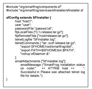
Figure 1. SFInstaller component
