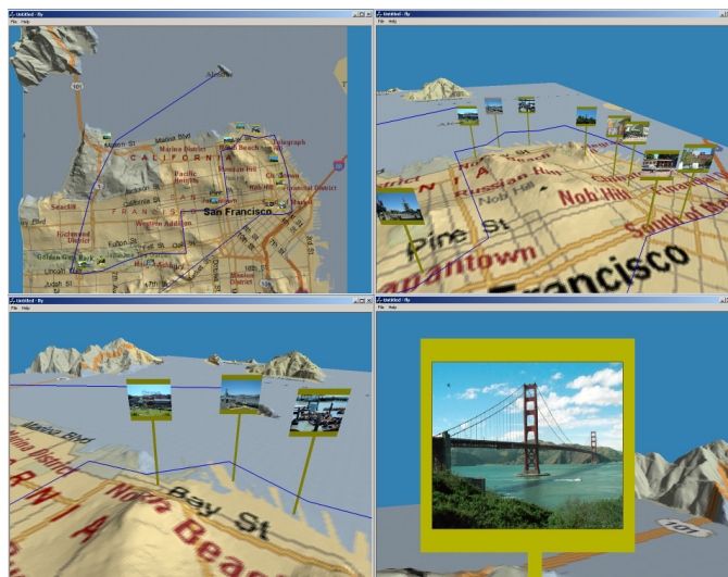
Fig. 2. Four views of a PEM flyby with a city map texture-mapped on a Digital Elevation Model background. The figure shows a simplified path traveled together with billboard representation of the digital media.
